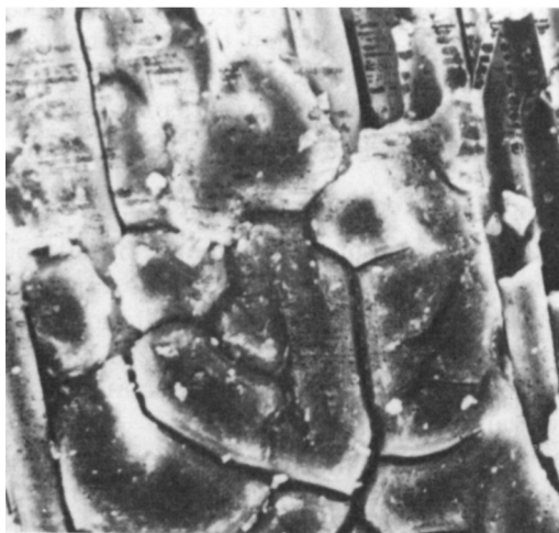
Fig. 20. Electron micrograph of TBBP-A-modified polyester containing 17% Br after eight months of natural weathering.
